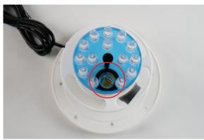
the diffuser plate should only be installed in this position
