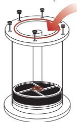
the reactor should be filled no more than 2/3 full to allow the media room to move around. With heavy or fine media, you may need to add less.
