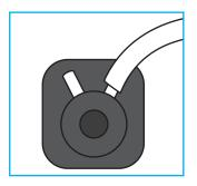
Connect the other end of the yellow airline tubing to one of the air inlets located on the pump venturi.
