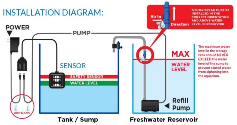
A "Drip Loop" should be arranged for EACH cord connecting the controller. The "Drip Loop" prevents water from traveling along the cord and coming in contact with the Sensor connections or the electrical receptacle.
